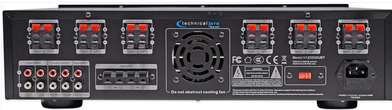
Figure 4.3: Rear panel of the H12X500UBT receiver, detailing speaker outputs, audio inputs, and antenna connections.
