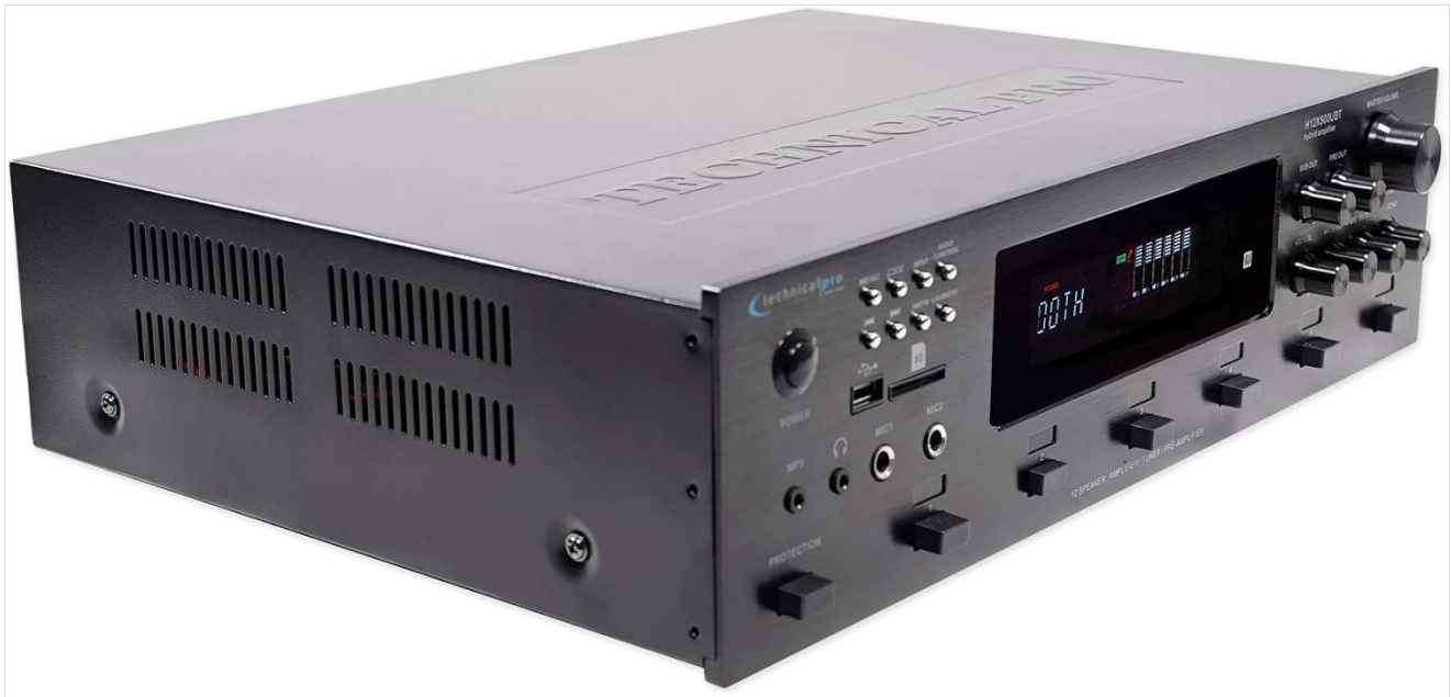
Figure 5.1: Receiver showing side ventilation for proper airflow.
