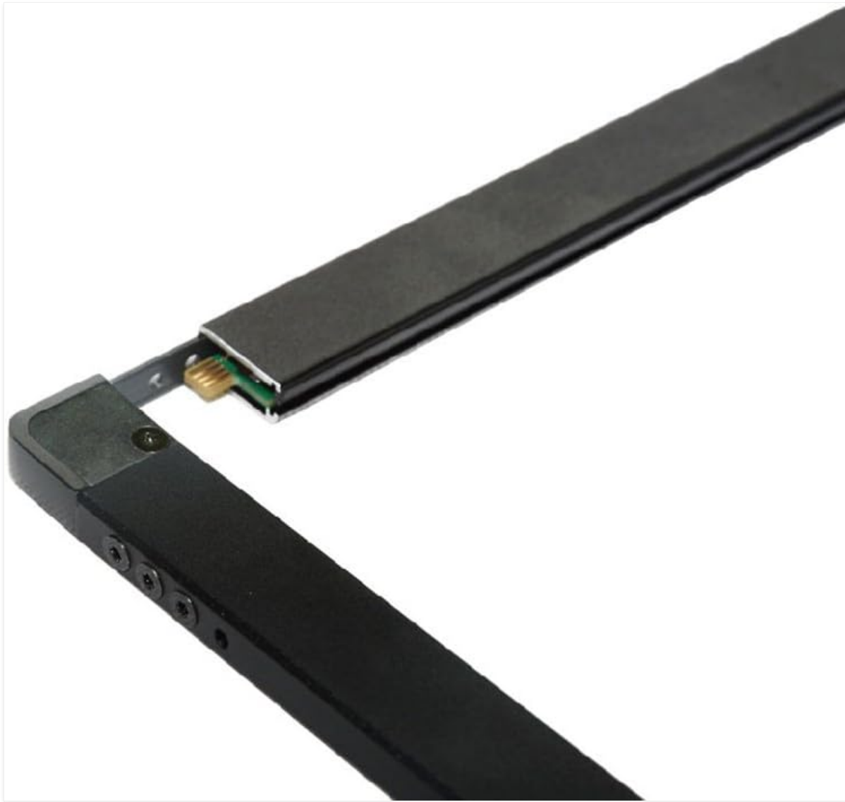
Figure 5: Detail of the corner connection, highlighting the internal circuit board and pins that connect the frame sections.
