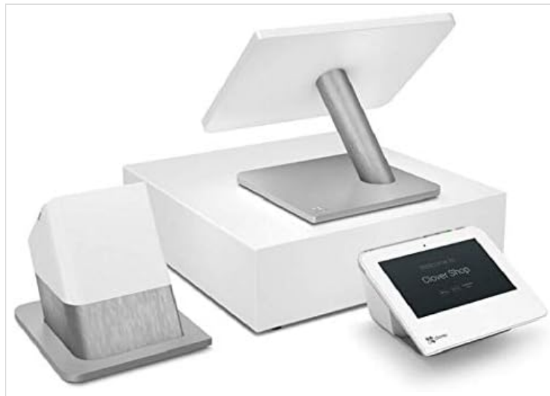
Figure 2.1: Overview of the Clover Station POS System components. This image shows the main merchant display unit, the customer-facing display with an integrated printer, and a separate cash drawer.
