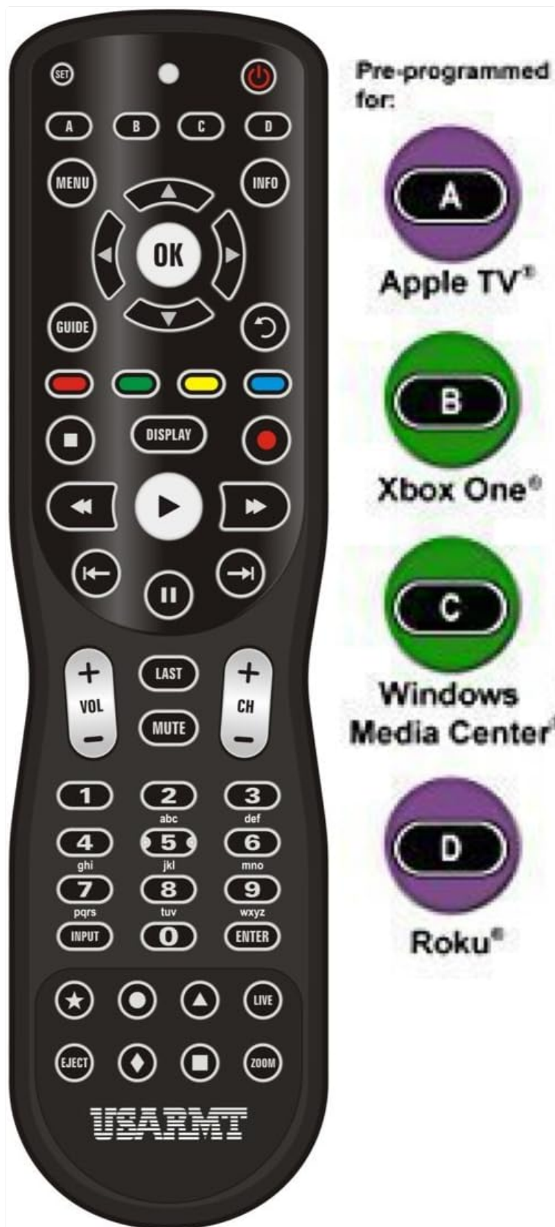
Figure 3: The top section of the remote highlighting the pre-programmed device selection buttons (A, B, C, D) and their corresponding devices.
