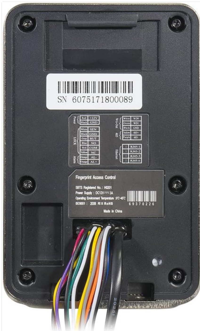
Image 4.2: Rear view of the PNI Finger 300 with wiring connections and product labels.
