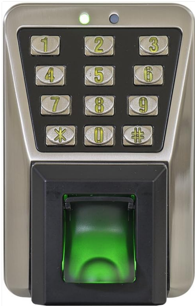
Image 4.1: Front view of the PNI Finger 300 showing the keypad, fingerprint scanner, and status indicators.
