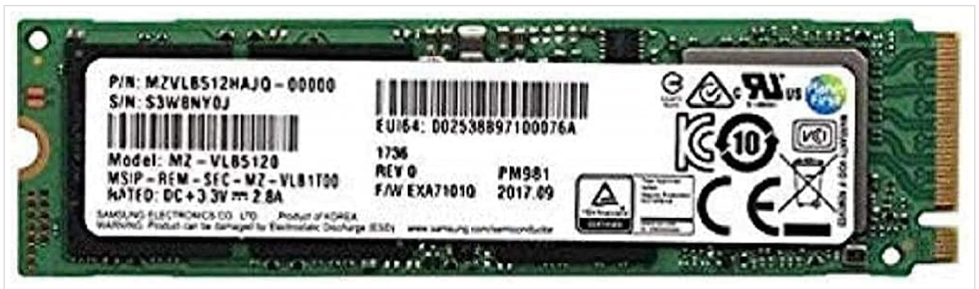
Figure 3.1: Samsung PM981 Polaris 512GB M.2 NVMe SSD. This image displays the physical appearance of the M.2 2280 form factor SSD, highlighting its compact design and component layout.
