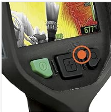
Figure 6: Detail of the FLIR K45 control buttons for navigation and mode selection.
