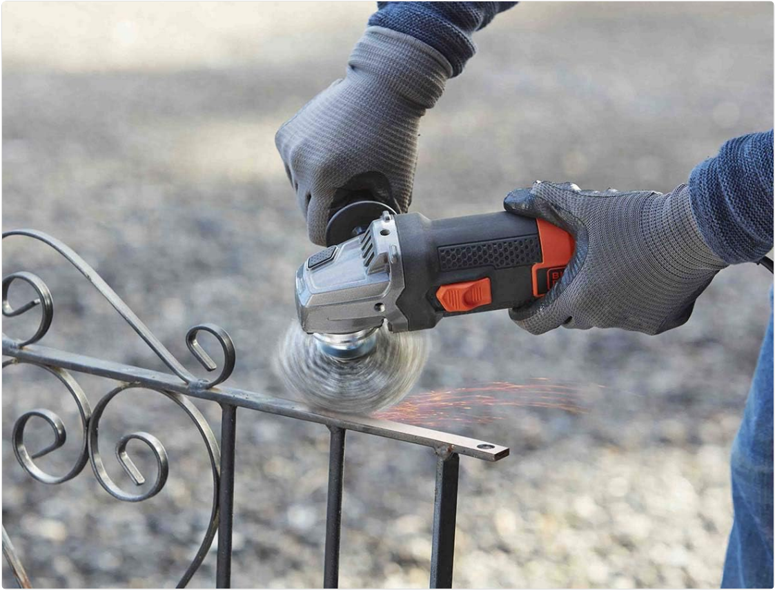
Figure 5: The angle grinder equipped with a wire brush attachment for surface preparation, such as rust removal.
