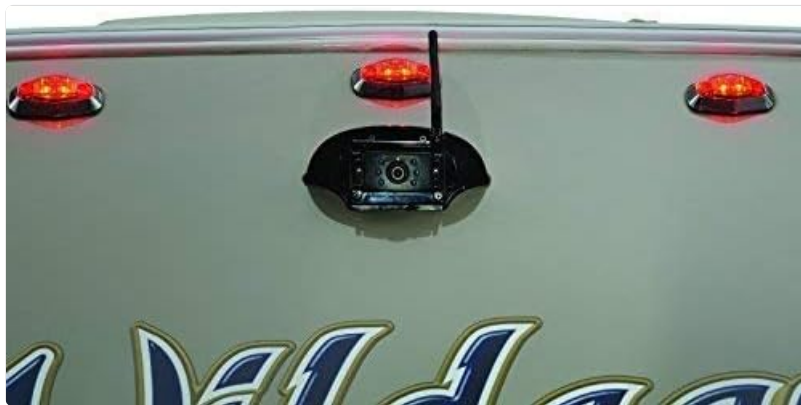
Figure 3.1: Rear sharkfin camera installed on an RV.
