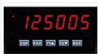
This image displays the front face of the PAXI0020 unit. It features a large, red seven-segment LED display at the top, currently showing '125005'. Below the display are five push-buttons: 'DSP' (Display), 'PAR' (Parameter), 'F1' (Function 1), 'F2'
