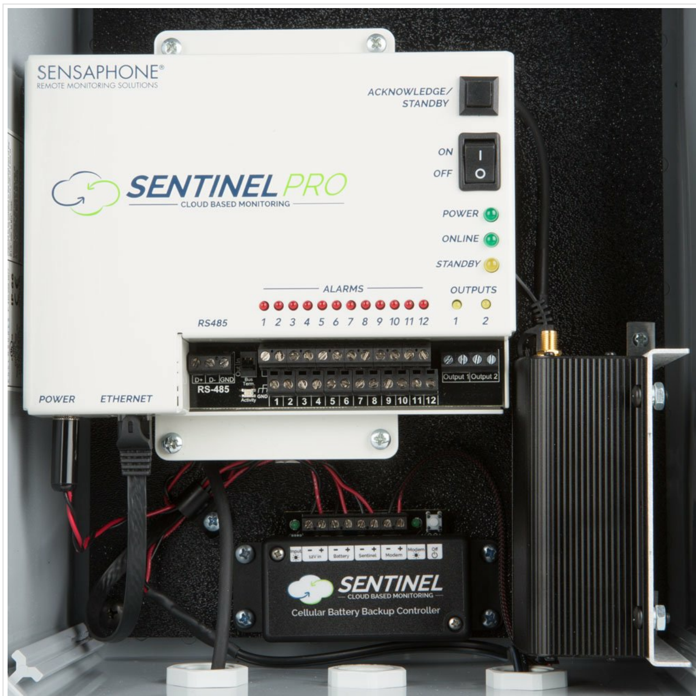
Figure 3.5: Detailed view of the Sentinel Pro's main board, showing sensor input terminals (1-12), RS485, Power, and Ethernet ports.
