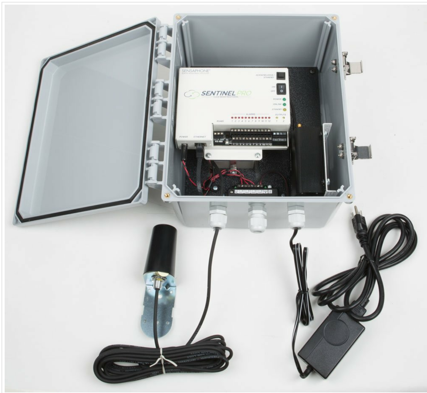
Figure 3.1: Sensaphone Sentinel Pro unit with cellular antenna and power adapter.
