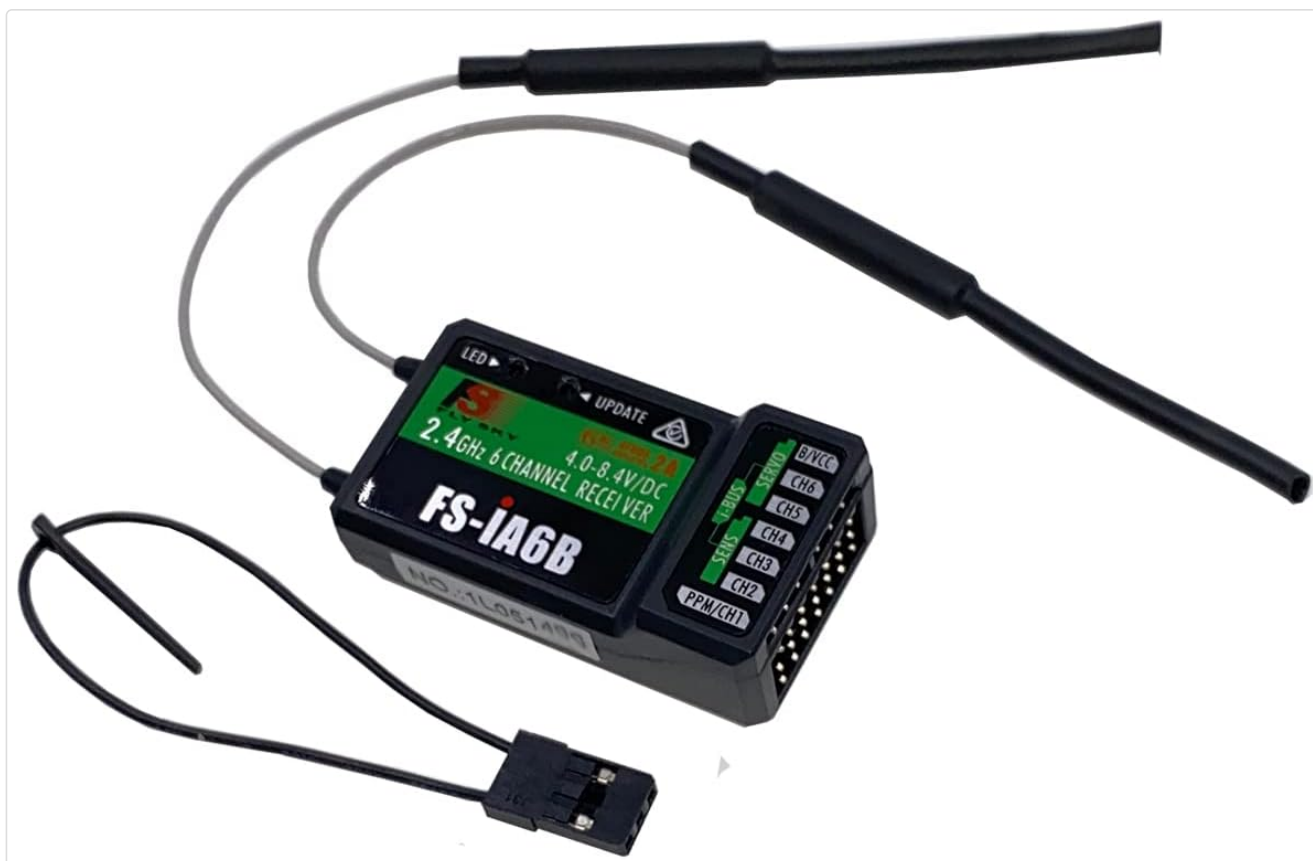
Figure 3.6: Close-up view of the FS-iA6B 6-channel 2.4GHz receiver.
