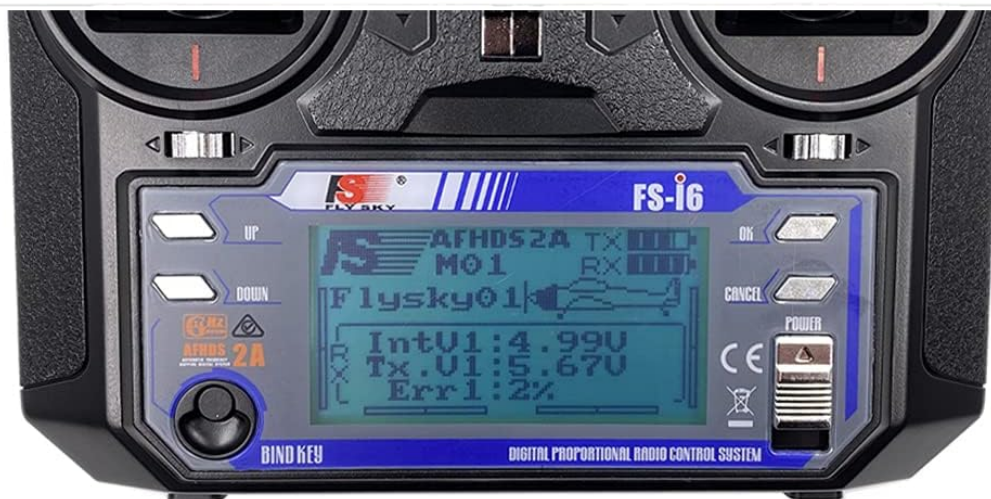
Figure 3.4: The FS-i6 features a dot matrix LCD backlit screen for clear display of operational data. It supports digital information in English or Chinese characters.
