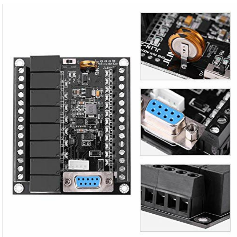
Figure 3.2: Close-up views of the DB9 communication port, backup battery, and input/output terminal blocks.
