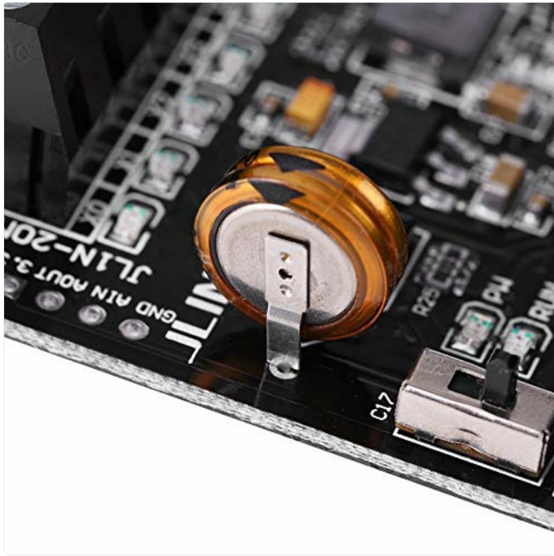
Figure 7.1: Close-up of the coin cell battery holder, indicating the location for battery replacement.
