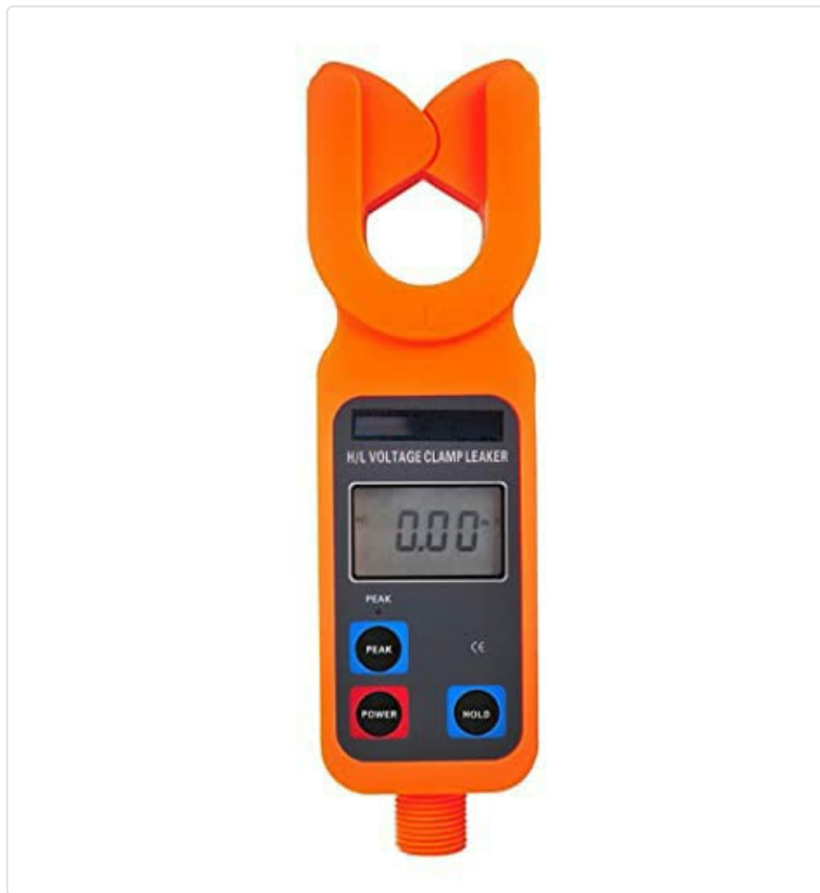
Figure 1.1: Front view of the ETCR910 Clamp Current Meter, showing the LCD display and control buttons.
