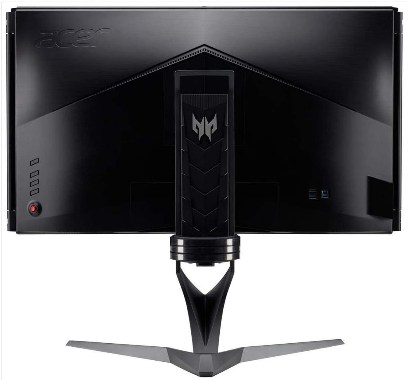
Image: Rear view of the Acer Predator X27 monitor, highlighting the DisplayPort, HDMI, USB, and power input ports.
