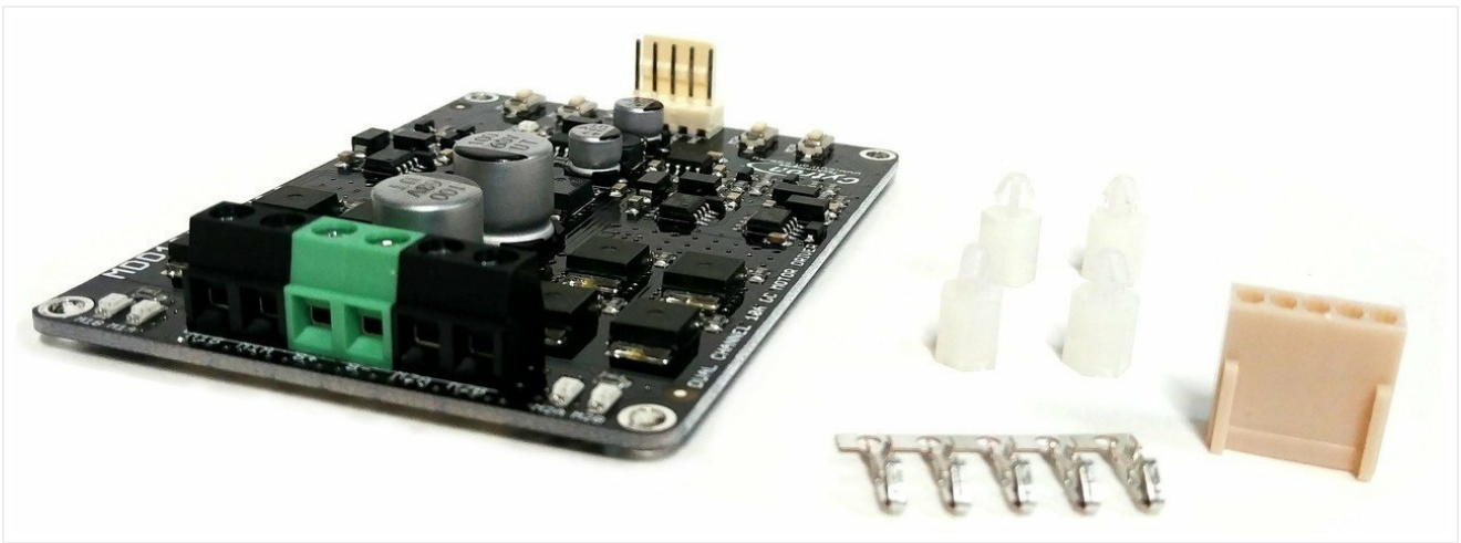
Figure 3.1: The Cytron MDD10A Dual Channel DC Motor Driver board shown with included accessories, including screw terminals, standoffs, and a header connector. This image provides a perspective view of the board and its components.
