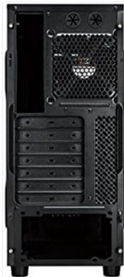
Image: Rear view of the Xigmatek Vanguard Plus PC case, highlighting the expansion slots and rear fan mounting area.
