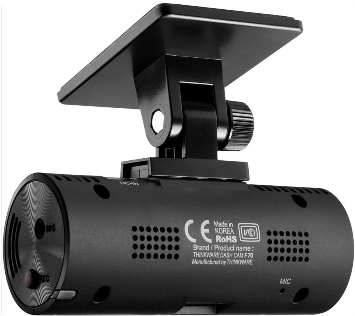
Image: The rear of the F70 dash cam showing its connection to the adhesive mount, ready for windshield attachment.
