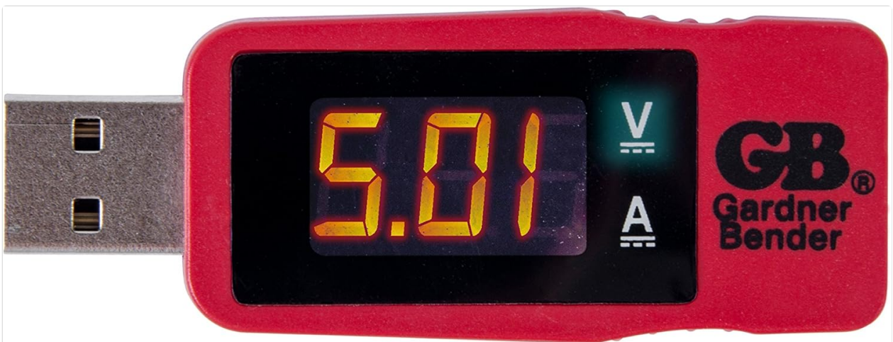
Image: The GUSB-3450 Multimeter's digital display showing a voltage reading of '5.01 V', indicating the measured voltage.
