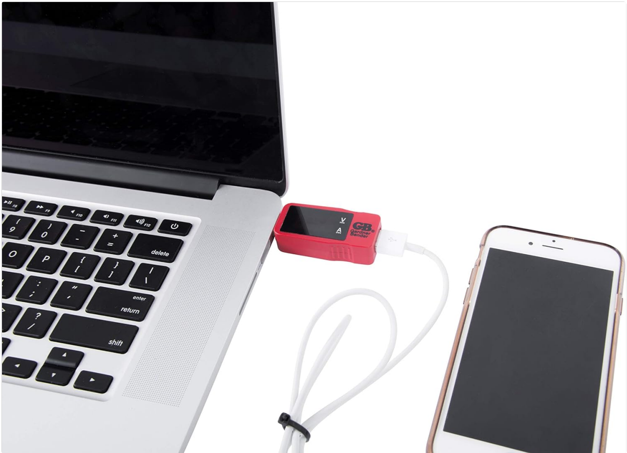
Image: The GUSB-3450 Multimeter connected to a laptop's USB port, with a charging cable extending to a smartphone, illustrating a typical setup.
