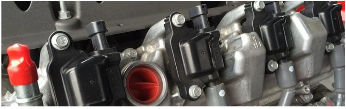
Figure 2: Typical engine bay view showing ignition coils. This image illustrates the general location of ignition coils, which cover the spark plugs in many modern engines.
