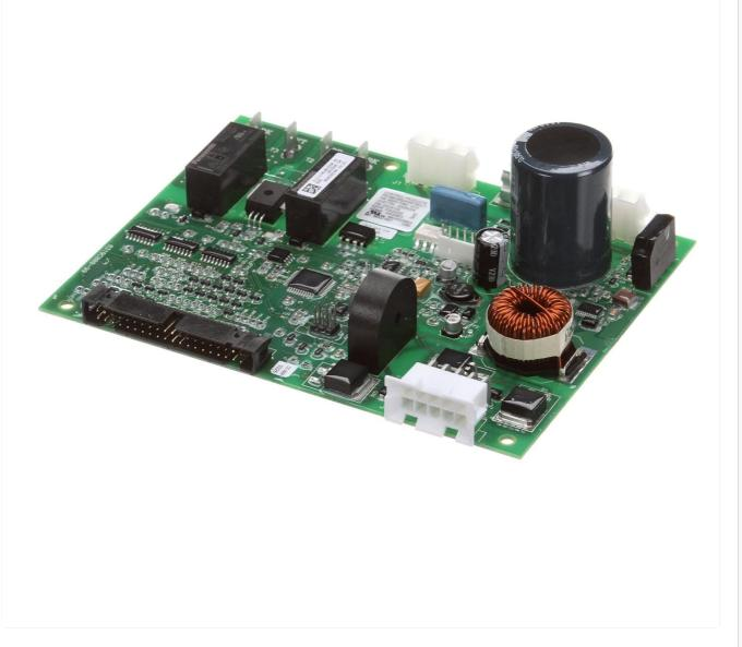
Figure 1: Front view of the Amana Menumaster 59004084 Main Control Board, showing various electronic components and connectors.
