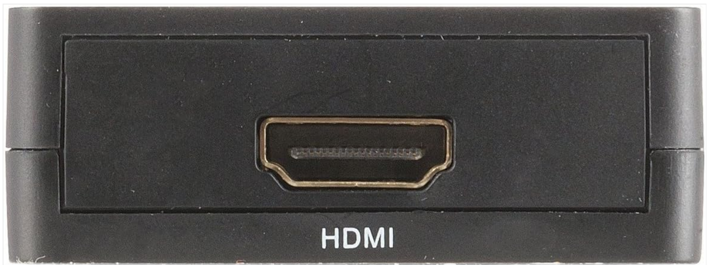
Image 2: Side view of the converter showing the HDMI output port. This port is labeled "HDMI" and is where the HDMI cable connects to your display device.
