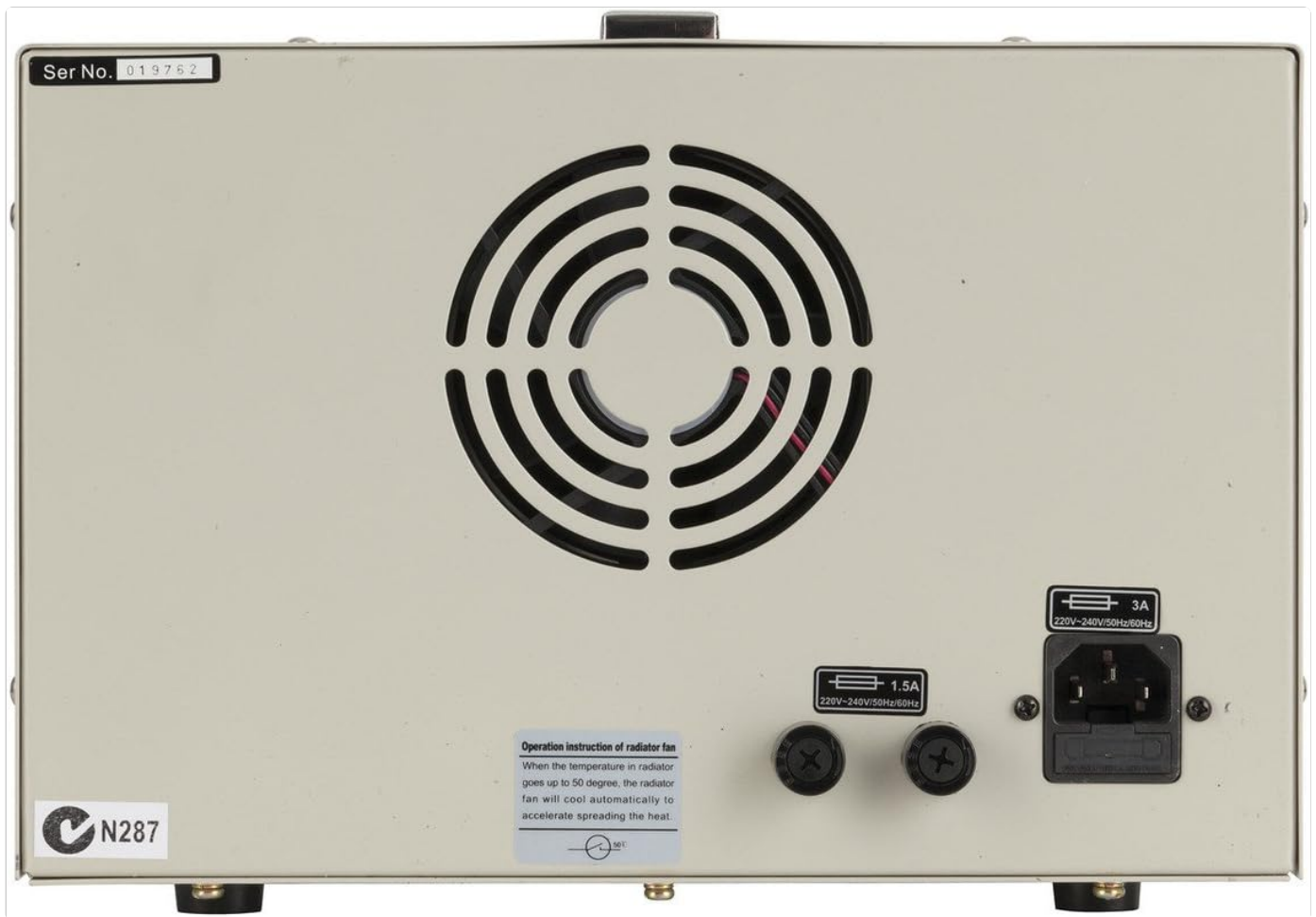
Figure 2: Rear view of the Powertech MP3087 showing the power input, fuse holder, and cooling fan.
