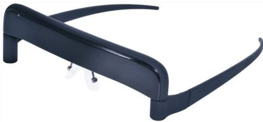
Figure 3.2: Angled view of the GlassOuse V1.4, highlighting the main body and temple arms.
