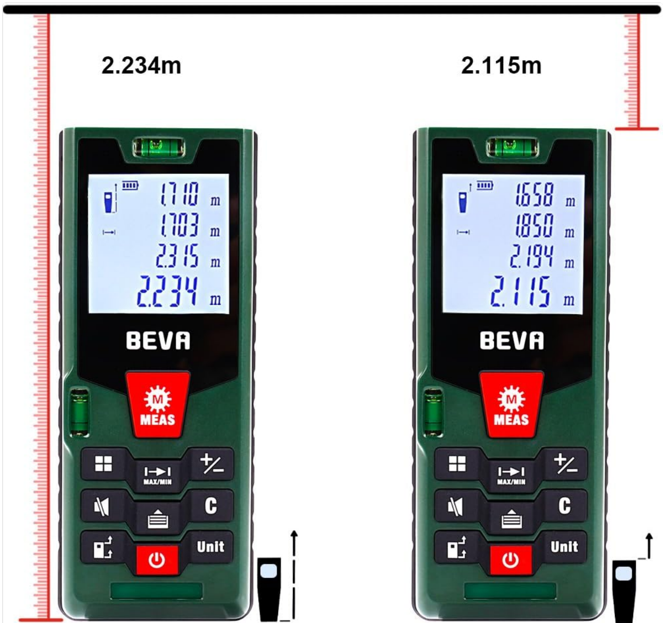
Image 5.1: Two BEVA Laser Measures demonstrating the difference between measuring from the rear reference point (left) and the front reference point (right). The display shows the measurement value relative to the chosen reference.
