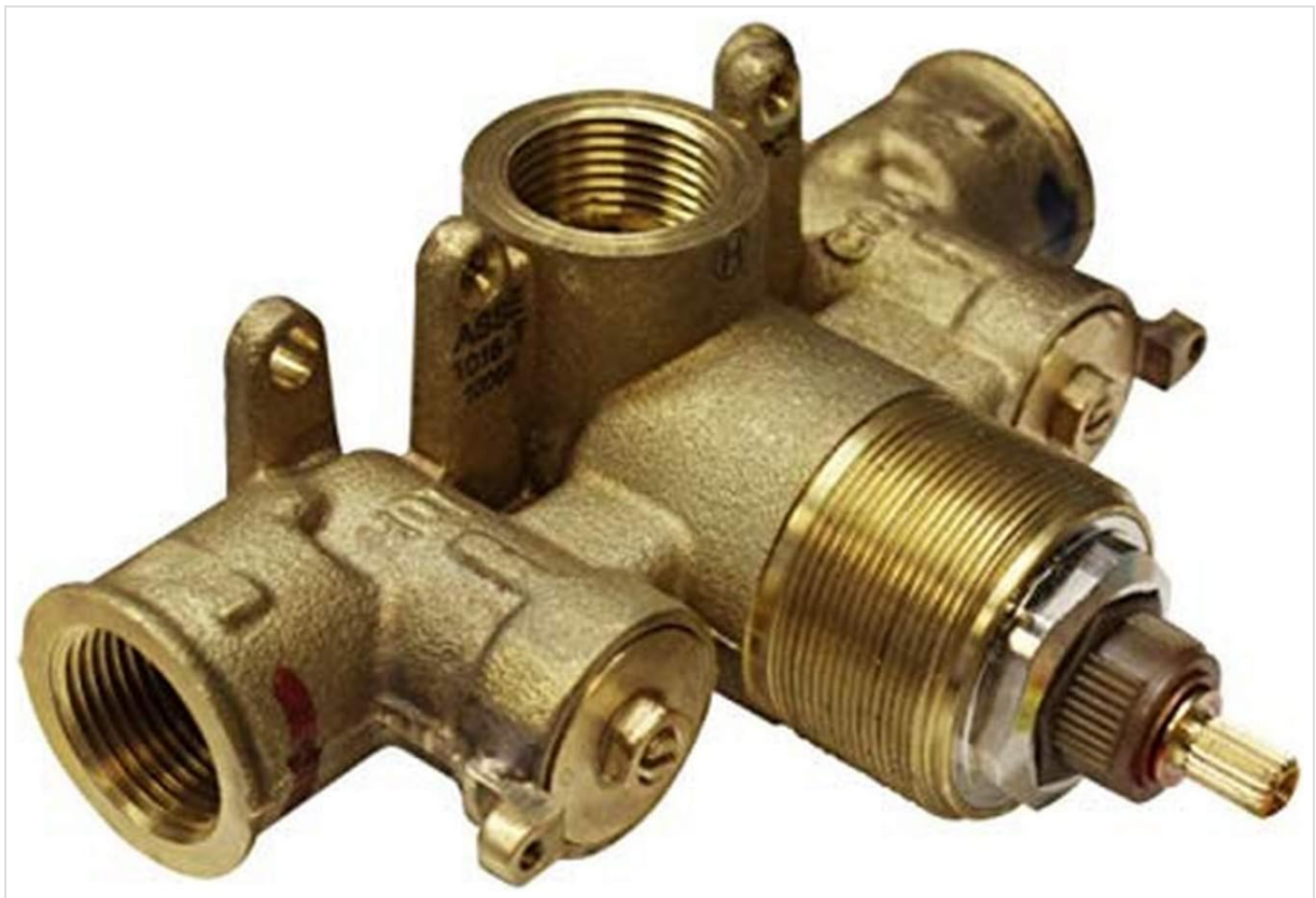
Figure 1: ROHL 1005N Thermostatic Rough Valve. This image displays the brass rough valve with threaded inlets and outlets, and the central thermostatic cartridge housing. Note the mounting tabs and the mud guard indicating installation depth.
