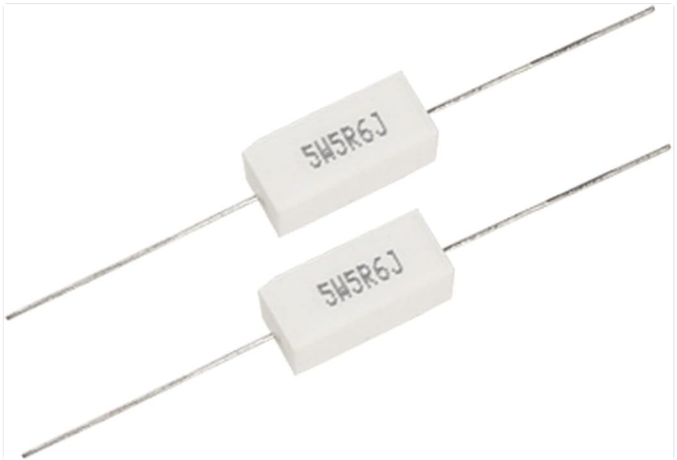
Figure 1: A pair of Aexit 5W 5.6 Ohm Ceramic Cement Resistors. These components are characterized by their white ceramic body and metallic axial leads, designed for through-hole mounting in electronic circuits. The marking "5W5R6J" indicates their power rating, resistance value, and tolerance.
