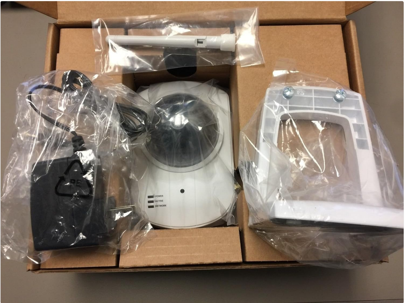
Figure 3.1: Package Contents. The image displays the SERCOMM RC8230D camera, its power adapter, and a mounting bracket, all neatly packed in their original packaging.
