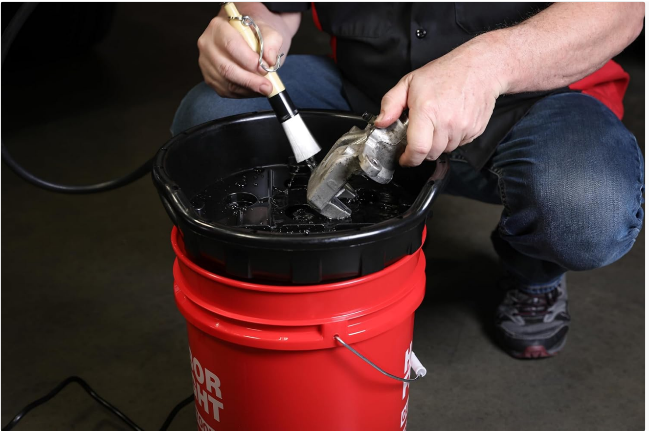
Image 5.1: Demonstrating the use of the parts washer to clean a component.
