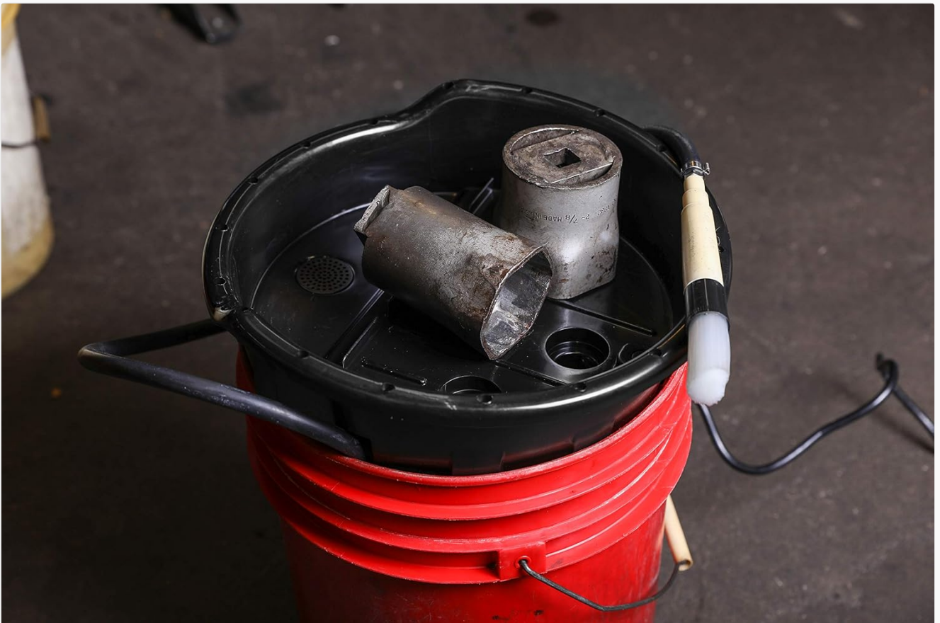
Image 5.2: Metal parts placed in the parts washer basin for cleaning.
