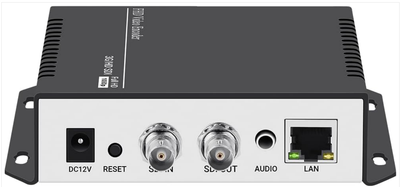
Figure 1.1: Front and Rear View of the URayCoder SDI to IP Encoder, showing DC12V power input, Reset button, SDI IN, SDI OUT, Audio input, and LAN port.
