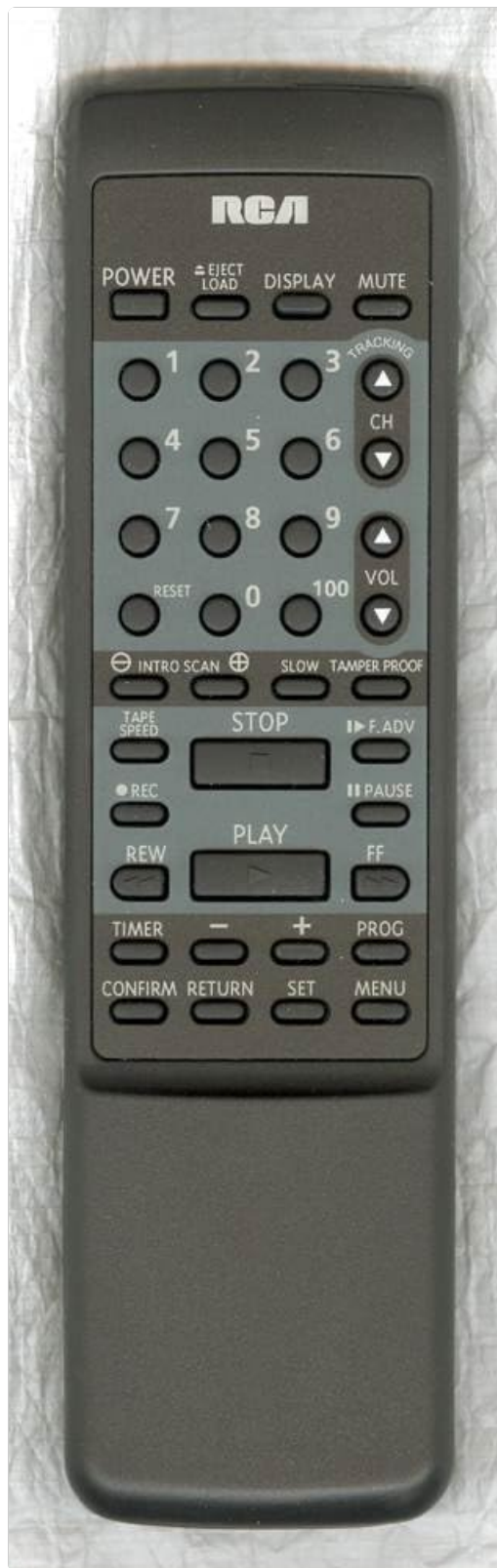
Figure 1: RCA OEM 228892 TV/VCR Combo Remote Control, front view showing all buttons. The remote is dark gray with light gray buttons. The RCA logo is at the top. Key sections include power/display/mute, number pad (0-9, 100, Reset), channel/volume controls, VCR transport controls (Stop, Play, Rewind, Fast Forward, Pause, Record, Intro Scan, Tape Speed, F.ADV, Tamper Proof), and function buttons (Timer, Minus, Plus, Program, Confirm, Return, Set, Menu).
