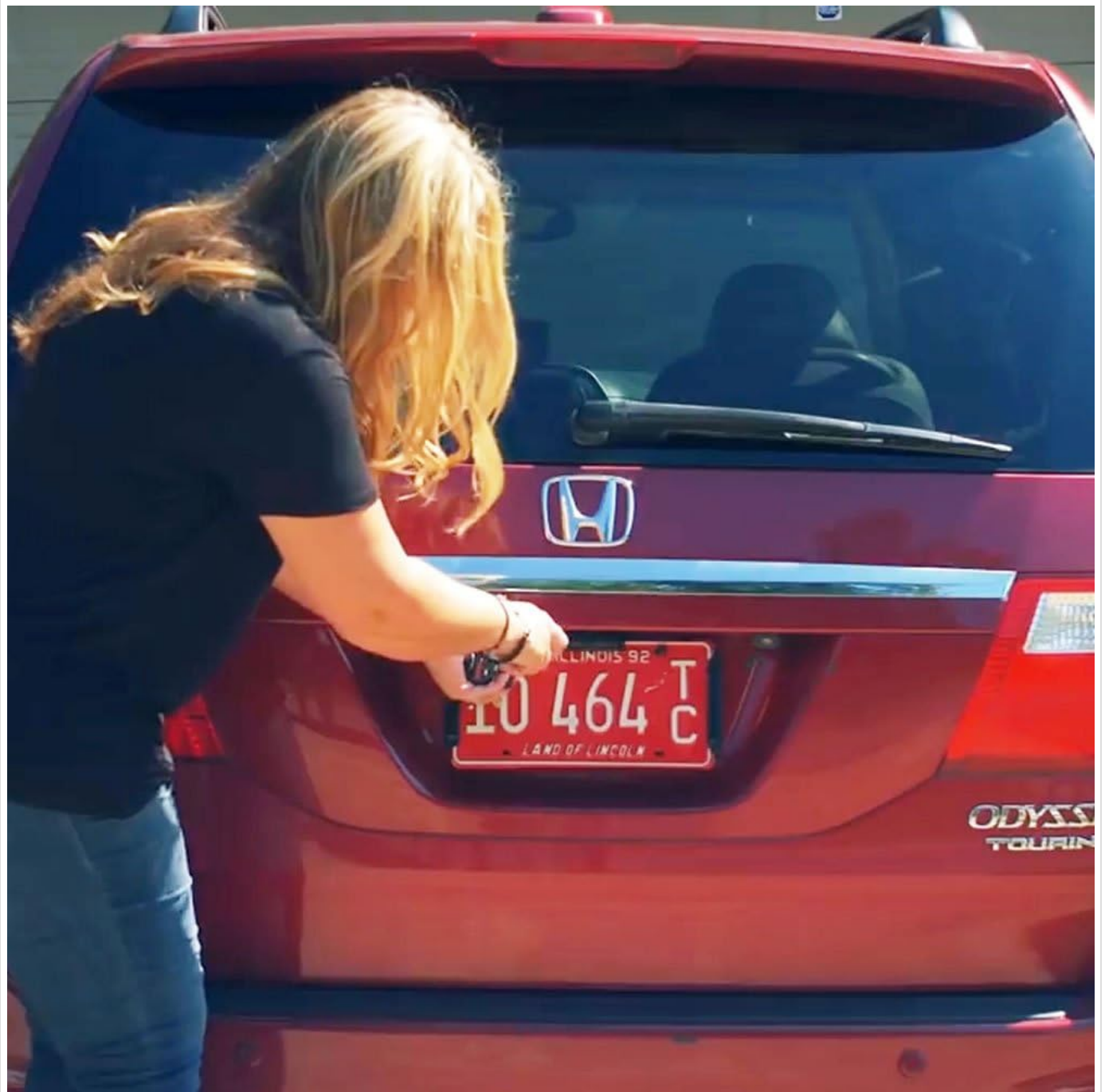
Image: A person installing the Whistler WBU900 backup camera by attaching it to the vehicle's rear license plate frame.
