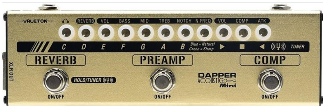
Figure 4: Top-down view of the pedal, showing the tuner's LED display indicating notes and tuning status.
