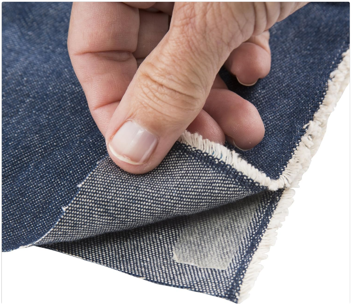
Image 3.2: The tape strip fully applied between two layers of denim fabric, creating a temporary hem.
