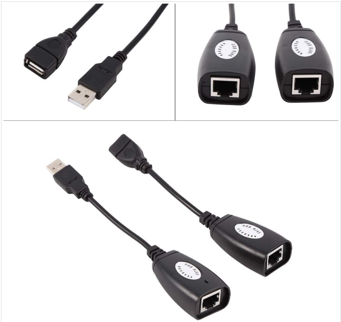
Image 2: Close-up view of the USB and RJ45 connectors on the extension adapter units.
