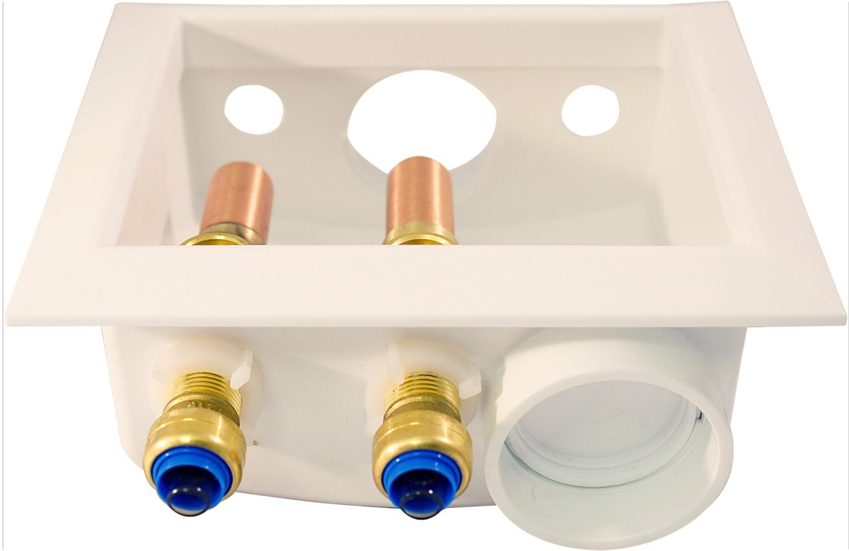
Figure 3: Bottom view of the outlet box, highlighting the push-to-connect inlets for hot and cold water supply lines. These fittings are compatible with copper, CPVC, PEX, and PE-RT pipes.
