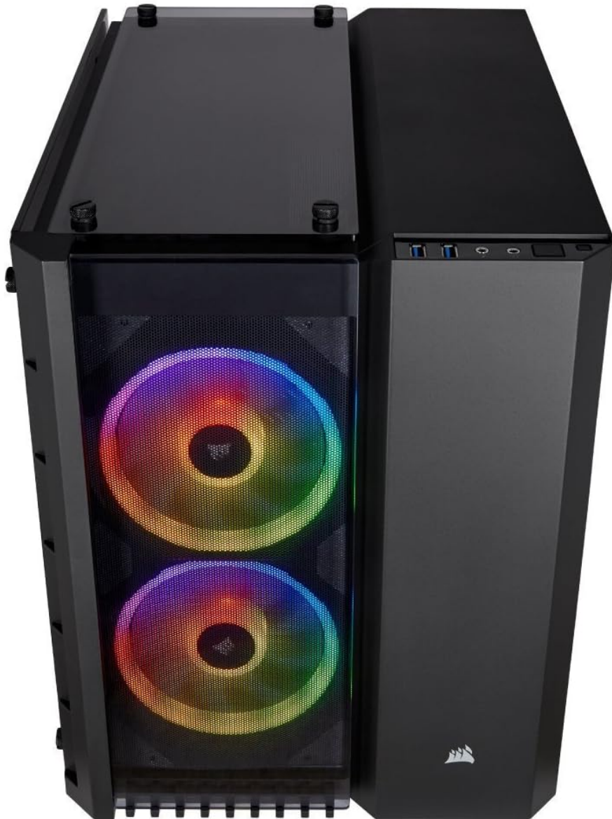
Figure 4.1: Front panel with visible RGB fans and magnetic dust filter.
