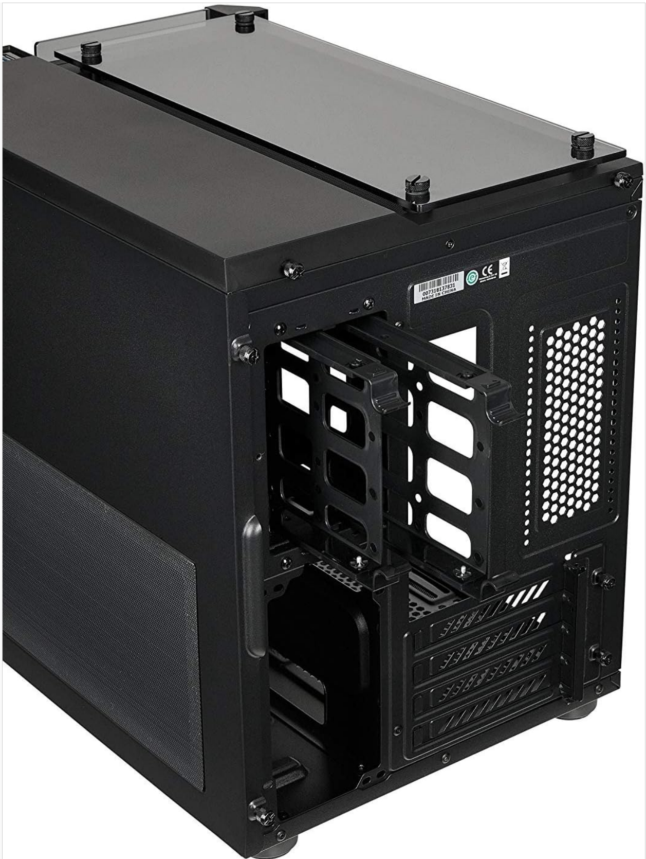
Figure 2.2: Rear compartment with hot-swappable hard drive trays for 2.5" and 3.5" drives.
