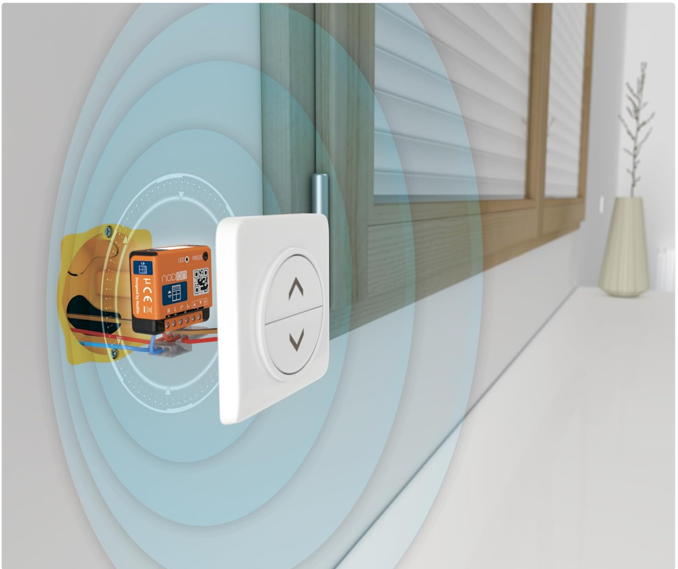
Figure 4.1: Example of NodOn module integration with a wall switch. This image visually represents how the module connects to a physical switch for local control, while also enabling wireless communication.
