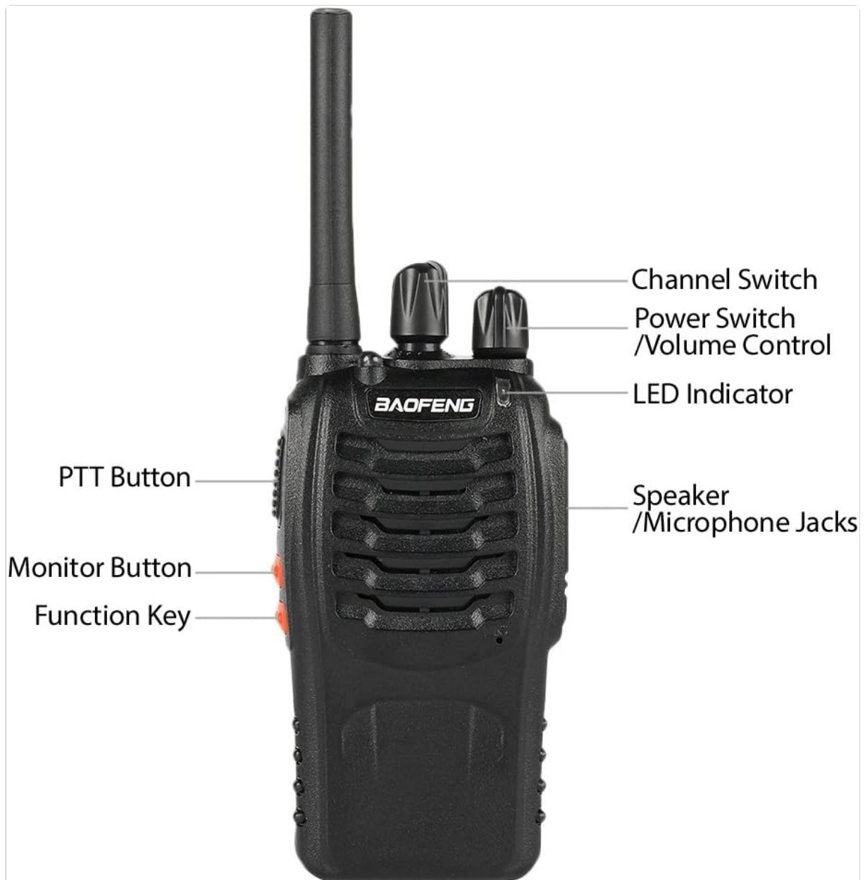
Image: Labeled diagram of the BAOFENG BF-88A radio components.
