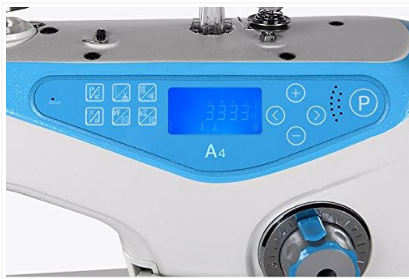
Figure 3.3: Close-up of the digital control panel with various function icons and display.
