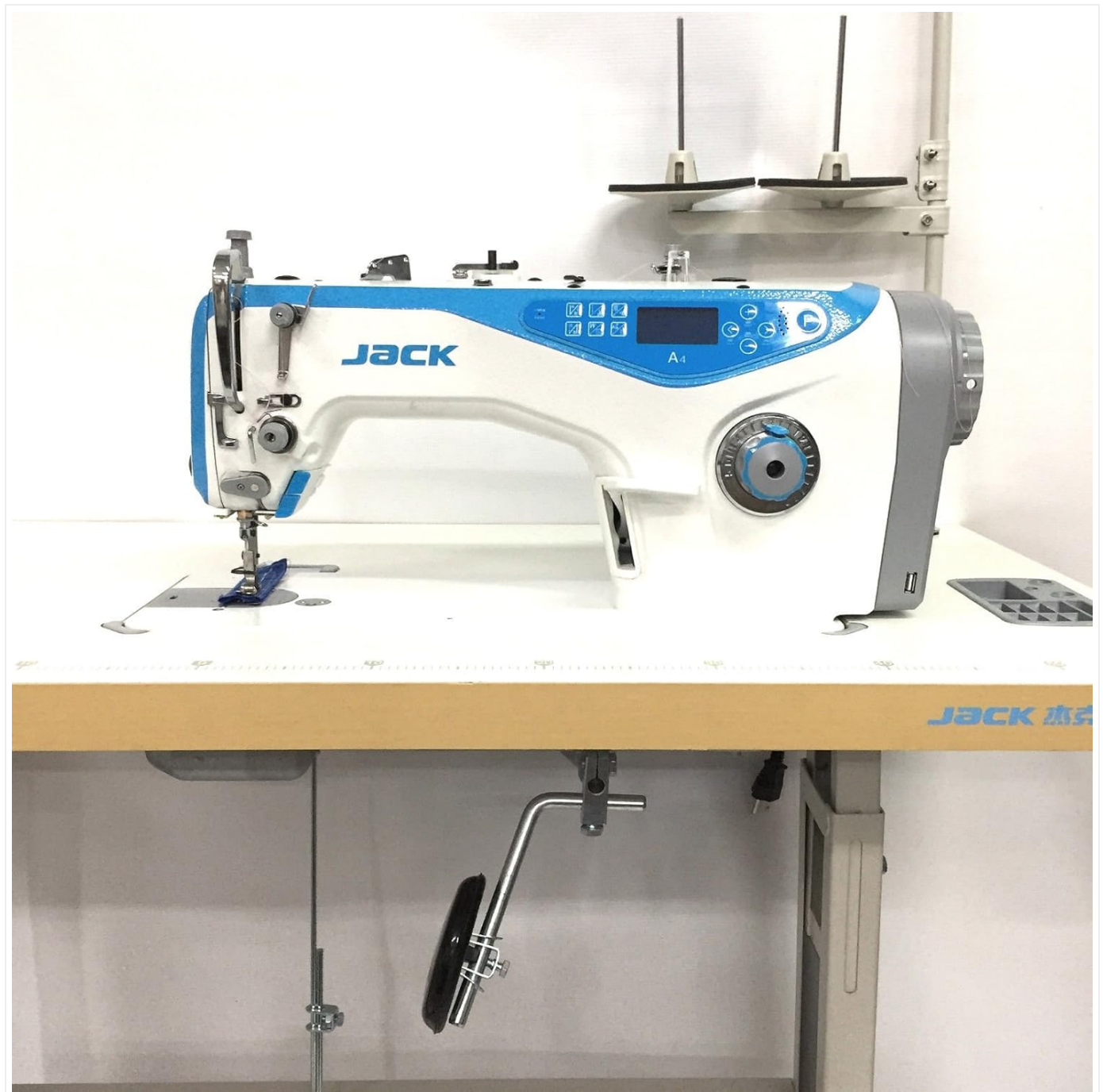
Figure 3.1: Overall view of the Jack A4 machine installed on a sewing table, showing the thread stands and integrated motor.
