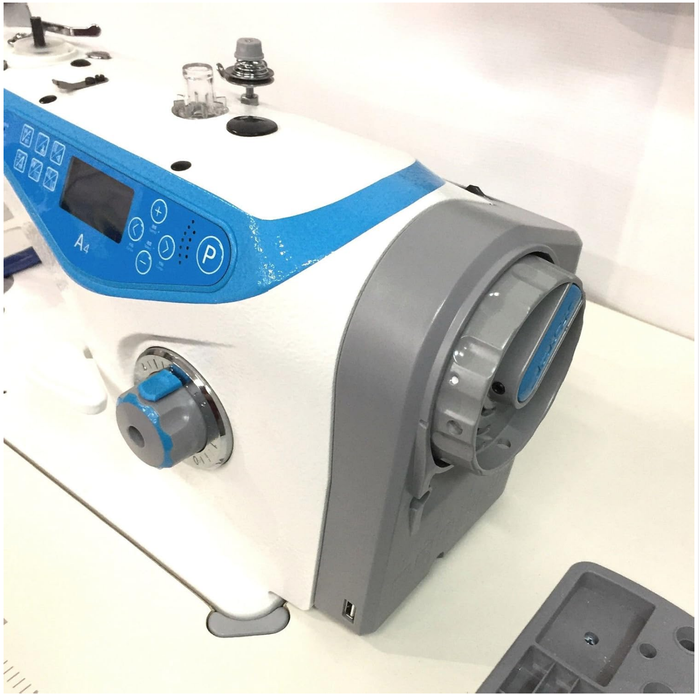
Figure 3.2: Detailed view of the machine's right side, highlighting the control panel, handwheel, and USB port.
