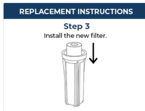
Figure 7: Replacement Instructions Step 3: Install the new filter.
