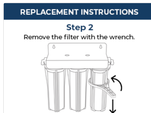
Figure 6: Replacement Instructions Step 2: Remove the filter housing with the wrench.
