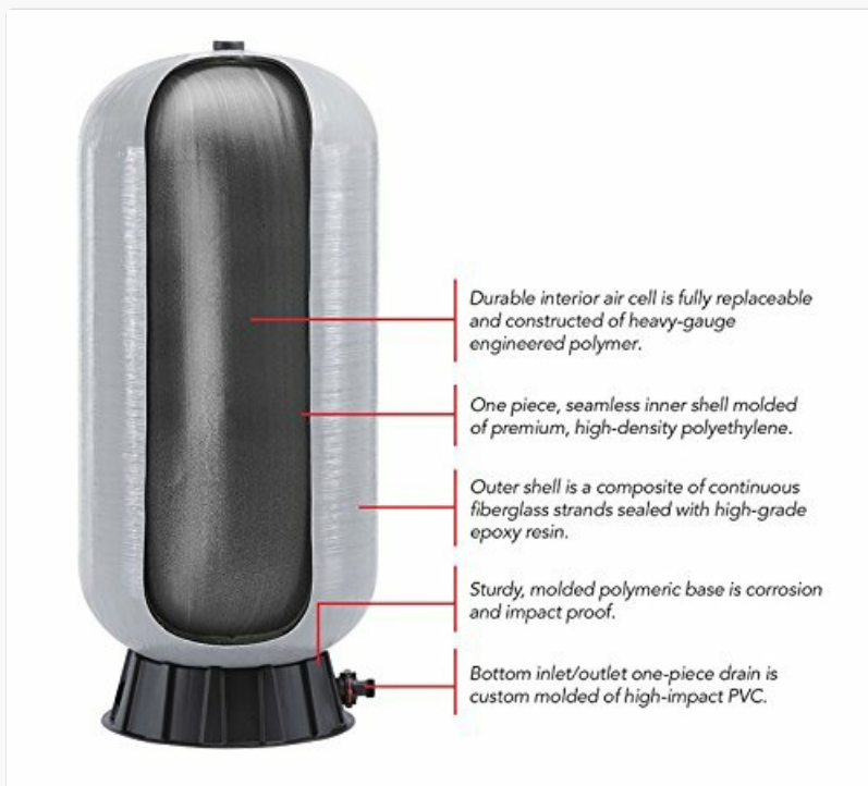
Figure 2: Cutaway diagram illustrating the internal components of the Wellmate WM-35 / WM0450 tank. This diagram highlights the durable interior air cell, seamless inner shell of high-density polyethylene, outer shell of continuous fiberglass strands sealed with epoxy resin, sturdy molded polymeric base, and the bottom inlet/outlet one-piece drain made of high-impact PVC.
