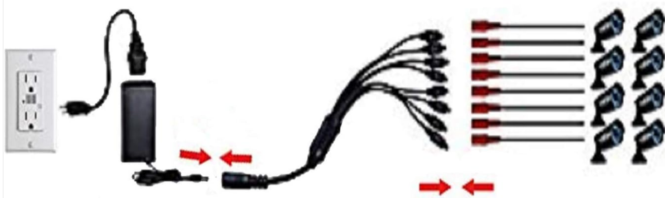
Image 4.1: Illustrative diagram showing the complete connection from wall outlet to adapter, then to the 8-way splitter, and finally to multiple cameras.
