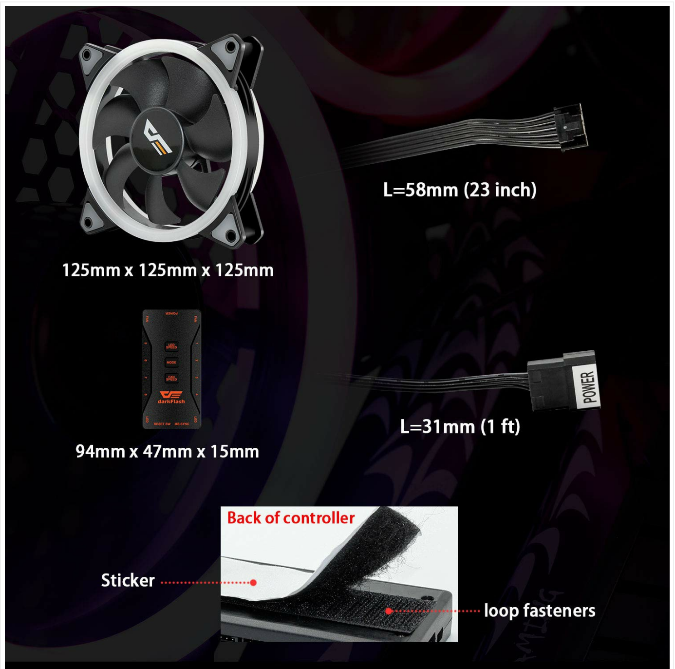
Image 4.4: Dimensions of the DR12 Pro fan and control hub, along with the adhesive backing for the hub.
