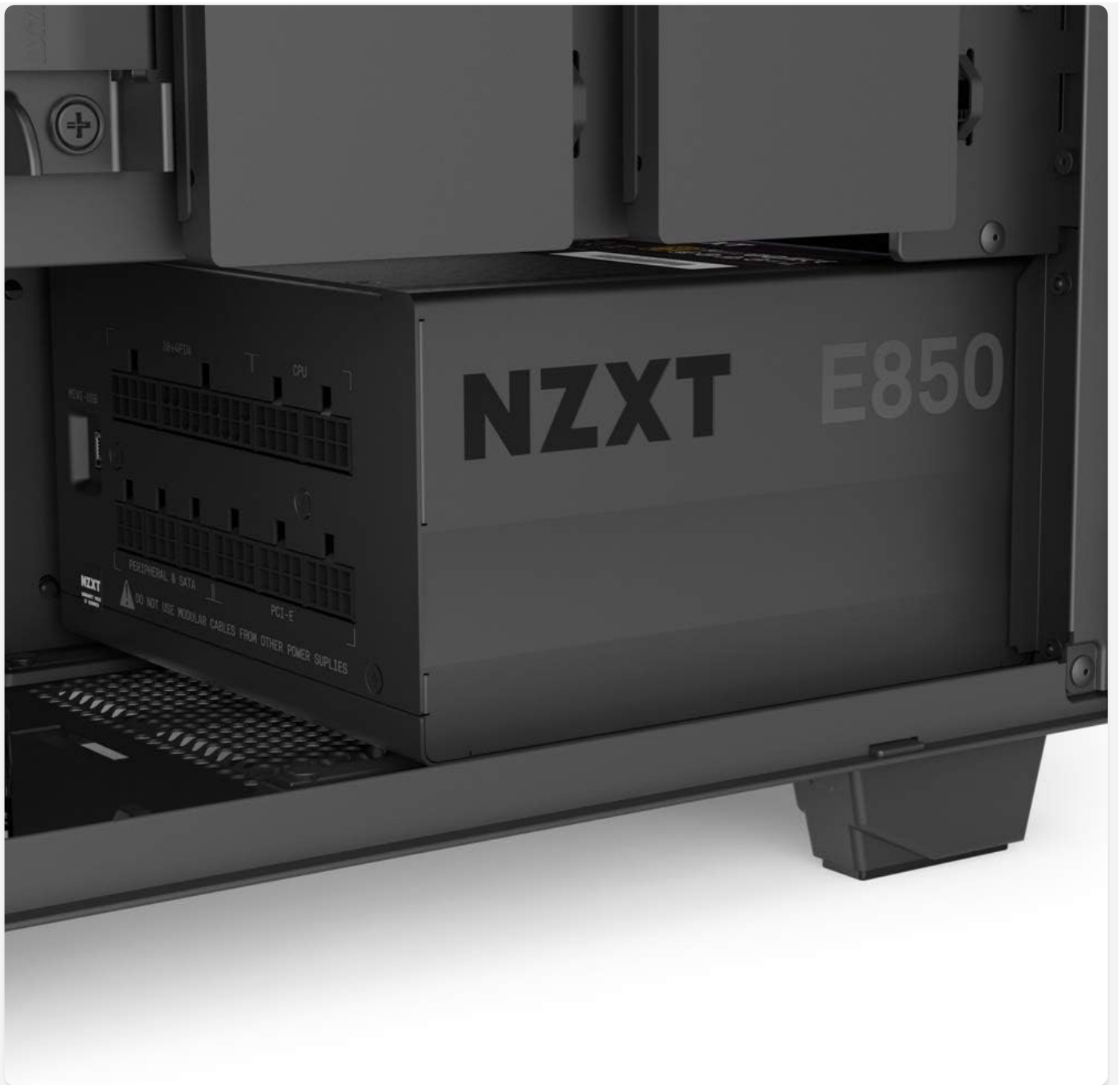
Figure 4: NZXT E850 PSU installed in a PC case, showing cable routing.
