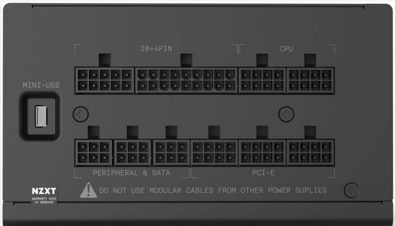
Figure 2: Modular ports on the NZXT E850 PSU. Connectors are clearly labeled for 20+4PIN (Motherboard), CPU, Peripheral & SATA, and PCI-E.
