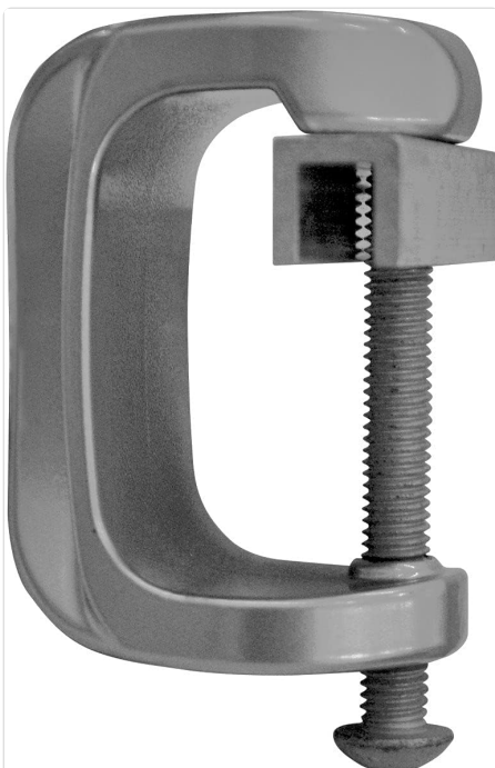
Figure 3.3: Detailed view of a C-clamp, which is used to secure the rack to the truck
