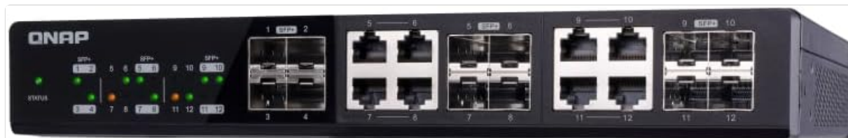
Figure 3.1: Detailed view of the front panel, highlighting the SFP+ and RJ45 combo ports, along with status indicators.
