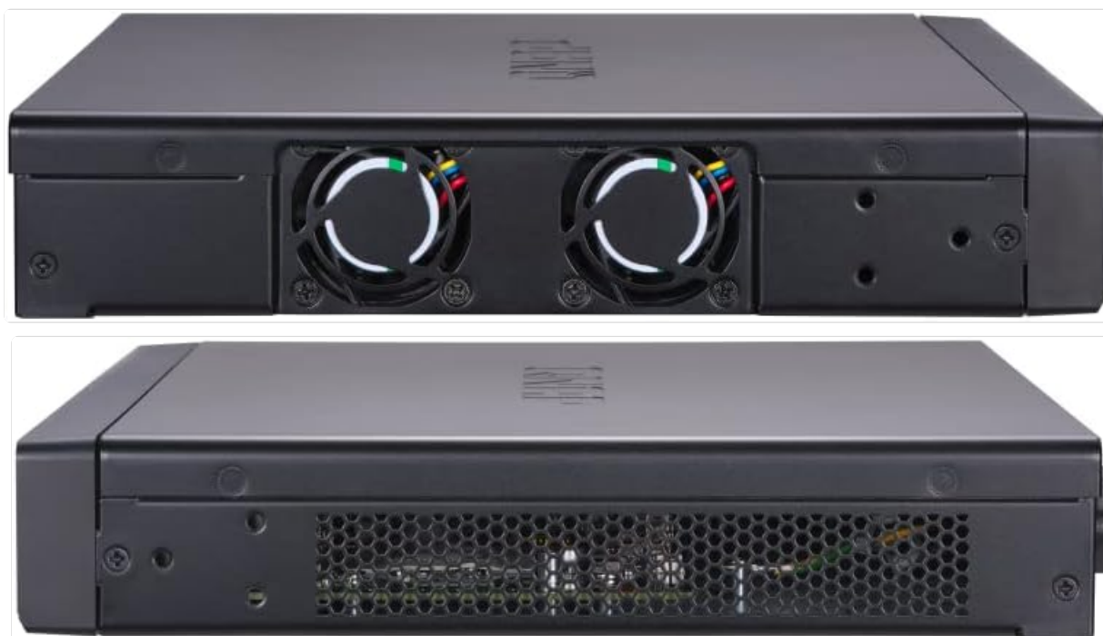
Figure 3.2: Side views of the switch, illustrating the cooling fans and ventilation grilles.
