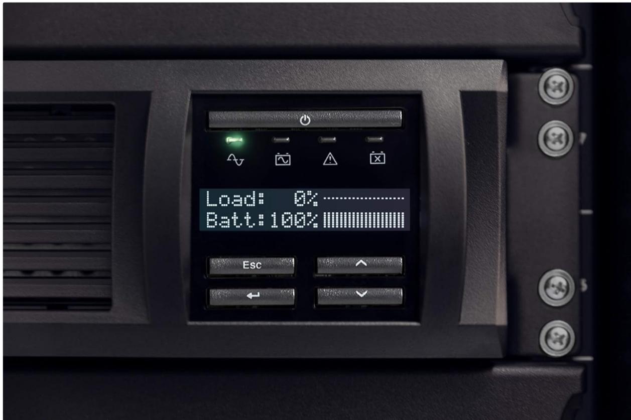
Figure 3.2: Close-up of the UPS LCD display, indicating 0% load and 100% battery charge.
