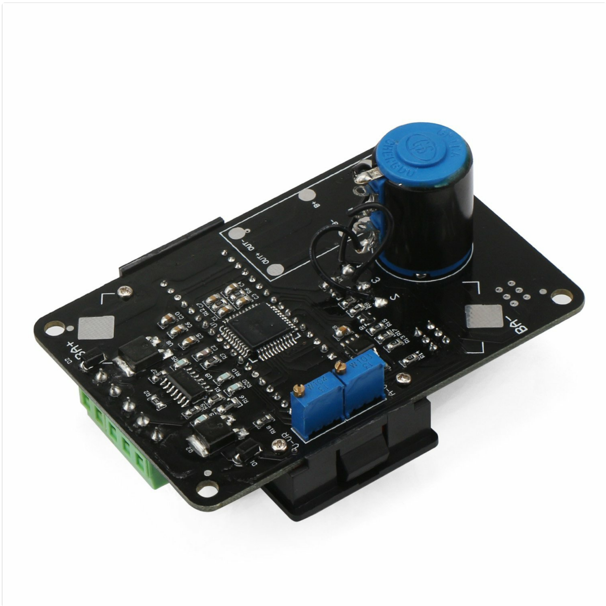
Image 5: Underside view of the DROK Signal Generator PCB, highlighting the two blue calibration potentiometers for current and voltage display adjustment.
