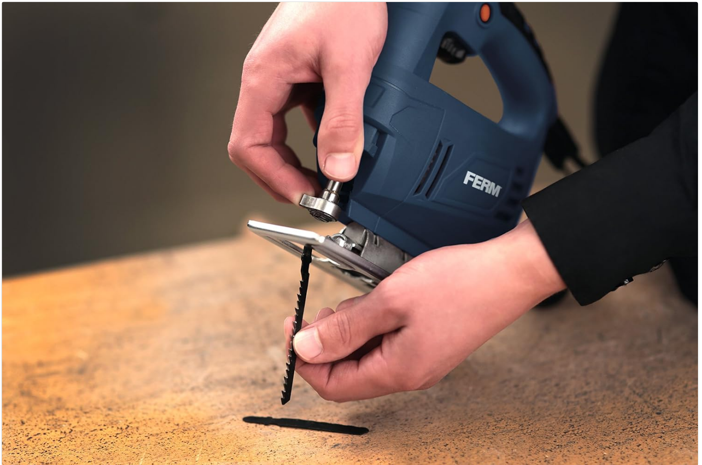
Figure 4.1: Illustration of a user installing a jigsaw blade into the tool's clamp mechanism.
