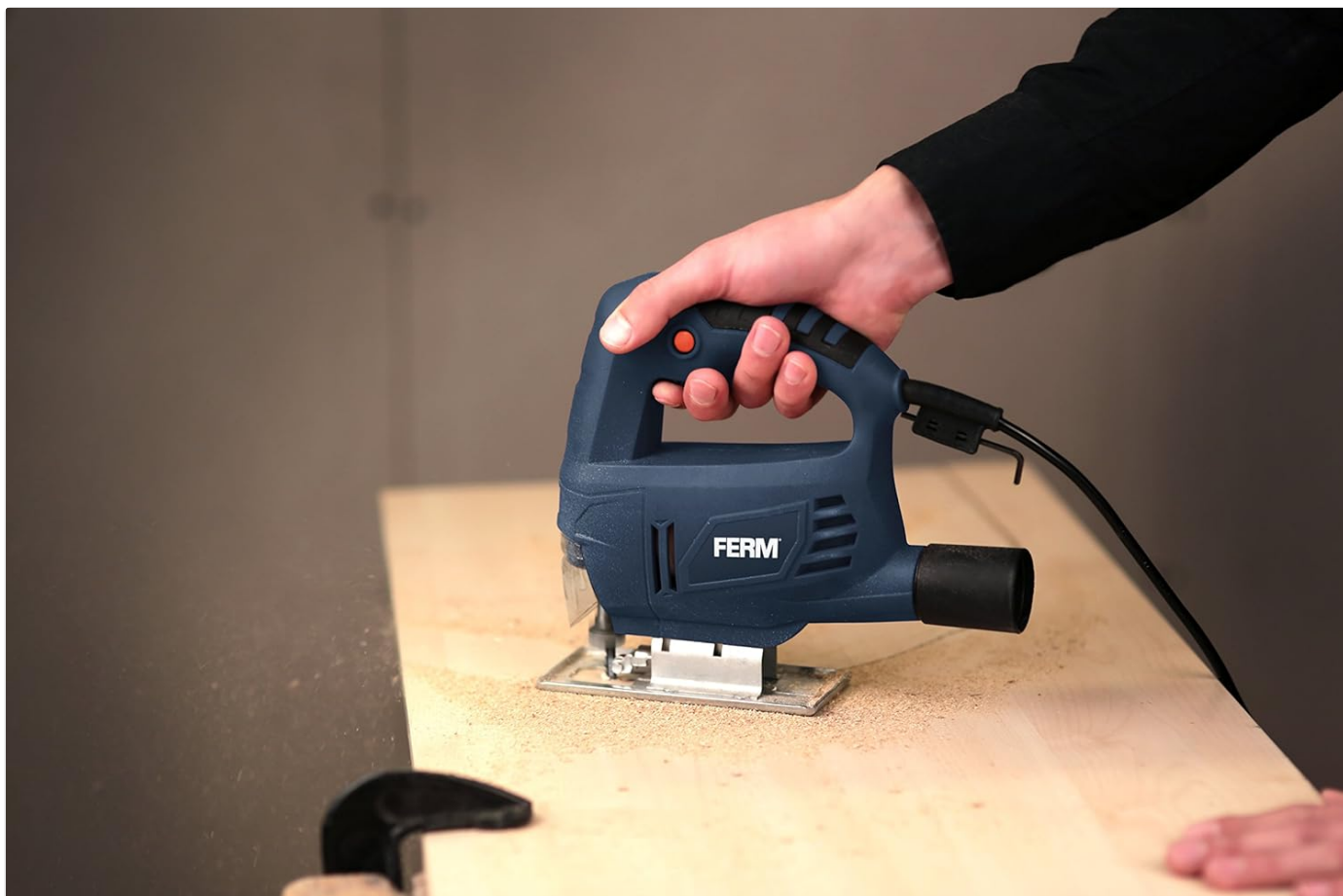
Figure 5.2: The FERM JSM1030 Jigsaw in action, cutting through a wooden panel, illustrating the dust generated during operation.
