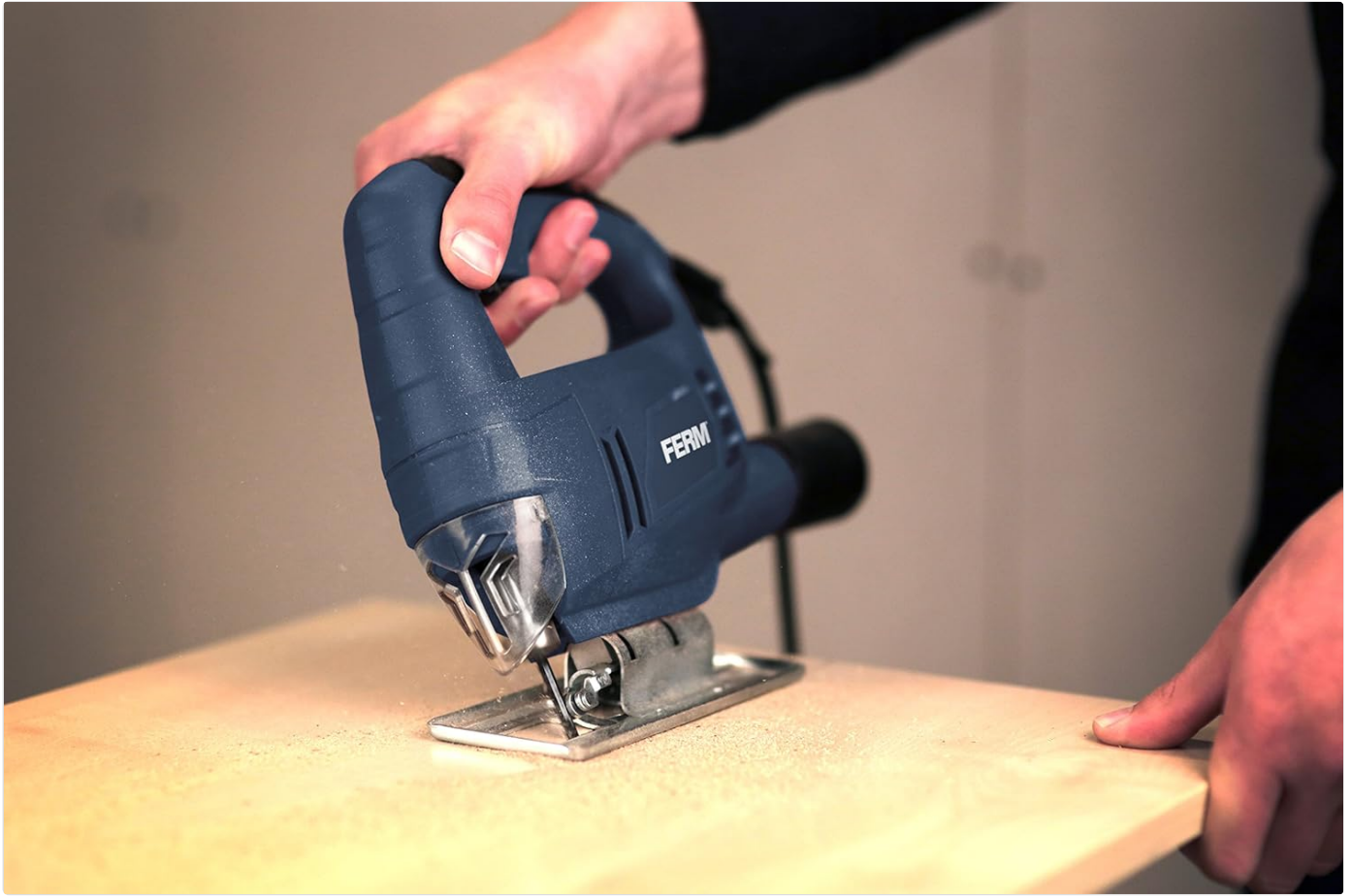
Figure 5.1: A user operating the FERM JSM1030 Jigsaw to cut a wooden board, demonstrating proper grip and positioning.
